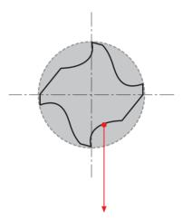
Improved chip disposal with the special flutes geometry and the irregular helix angle.
